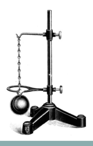
**Gravesande's ring** is a simple experiment used to demonstrate thermal expansion.
